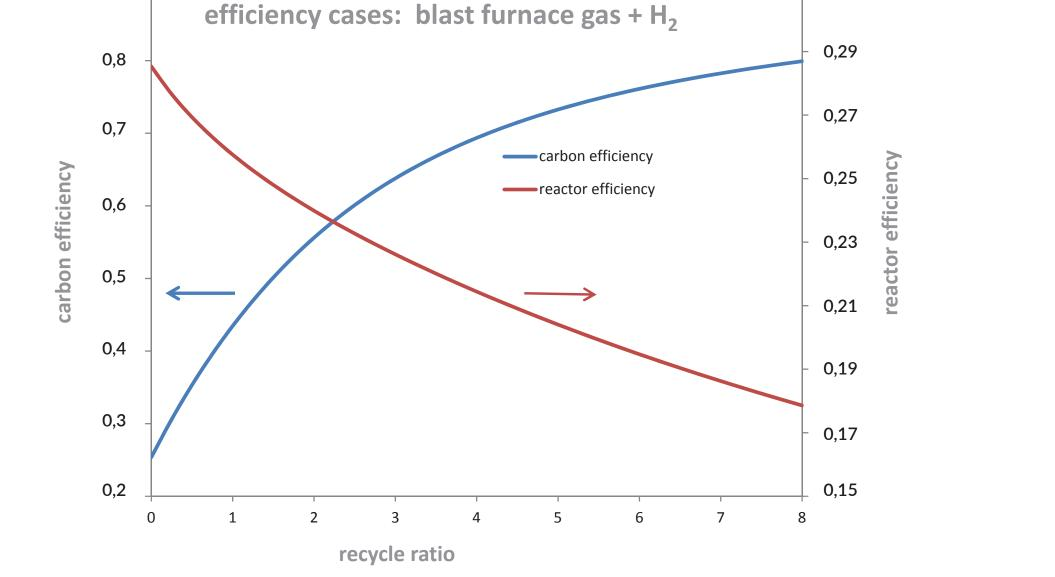
Simulation of a large scale methanol process with  $H_2$  enriched blast furnace gas as syngas source
